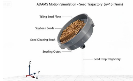
Figure 7 ADAMS motion simulation seed trajectories ( n = 15 r/min)
